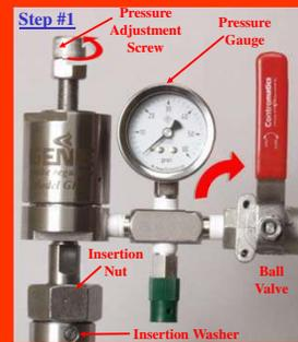
•Rotate the pressure adjustment screw fully counter-clockwise (unscrew it) until it rotates freely
