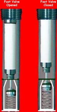
A stainless steel spring provides the initial upward force to close the foot valve. The process pressure provides additional force after the foot valve is closed.
